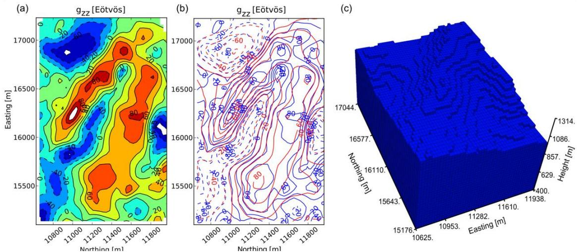
**Figure 4** Application to real FTG data. (a)  $g_{zz}$  component data used in the preliminary inversion. (b) Measured  $g_{zz}$  data in blue lines and  $g_{zz}$  data predicted by the inversion in red lines. (c) Interpretative model mesh including the topography of the region.
