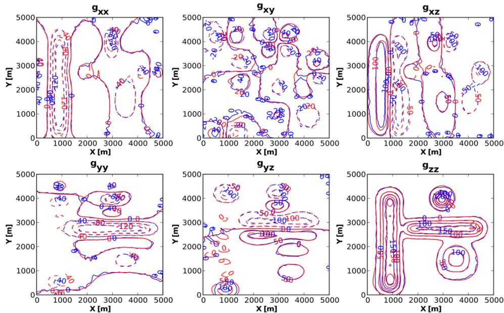
**Figure 2** Test using noise-corrupted synthetic FTG data. Synthetic data shown in blue lines and data predicted by the inversion in red lines.
