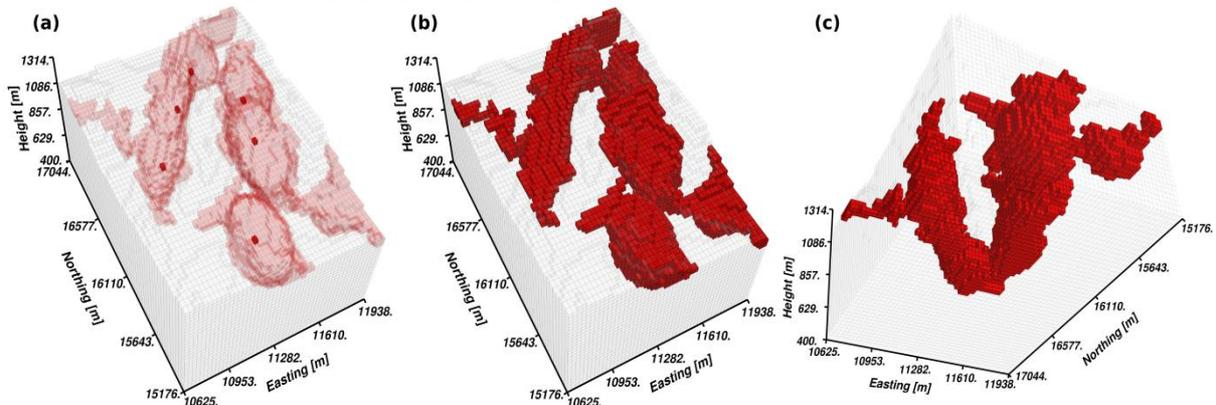
**Figure 5** Inversion result from the application to real FTG data. (a) Dark red cells represent the seeds provided to the inversion algorithm while light red cells represent the inversion result. (b) Top view of the inversion result. (c) Bottom view of the inversion result. Only prisms with positive density contrast of  $0.83 \text{ g.cm}^{-3}$  are shown.
