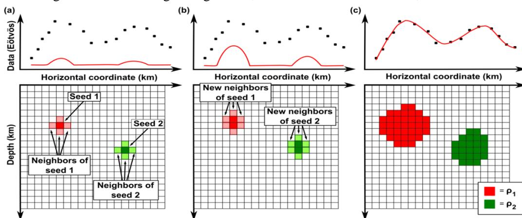
**Figure 1** 2D sketch of three stages of the algorithm. (a) Starting configuration using two seeds, one shown in dark red and the other in dark green. The neighbours of the red and green seeds are shown in light red and light green, respectively. (b) State of the solution after the first iteration. (c) The final result of the inversion after the algorithm stops showing compact bodies.
