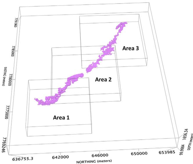
**Fig. 15.** Perspective view of the estimated density-contrast distribution (in pink) by inverting the six components of the gravity-gradient data shown in Fig. 8. This estimate retrieves the iron-ore body over the southern flank of the Gandarela syncline in Quadrilátero Ferrífero (Brazil).
