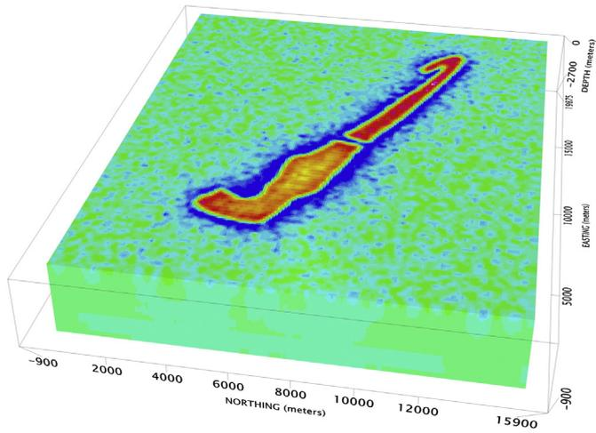
**Fig. 3.** Perspective view of the estimated density-contrast distribution by inverting the  $g_{zz}$  – component of the gravity gradient tensor (Fig. 2f) through the depth-weighting smoothing inversion.
