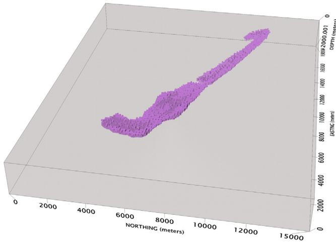
**Fig. 5.** Perspective view of the estimated density-contrast distribution by inverting the  $g_{xx}$ -,  $g_{xy}$ -,  $g_{xz}$ -,  $g_{yy}$ -,  $g_{yz}$ - and  $g_{zz}$ - components of the gravity gradient tensor (Fig. 2) through the planting anomalous density inversion.
