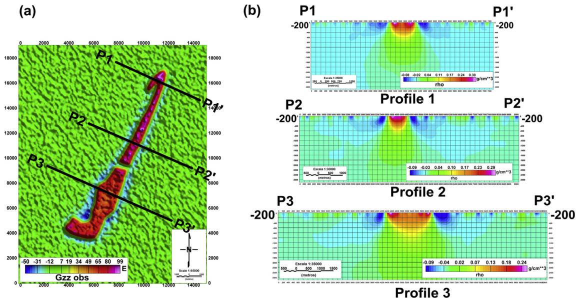
**Fig. 4.** (a) The observed  $g_{zz}$  – component of the gravity gradient tensor (Fig. 3f). The black lines P1–P1', P2–P2' and P3–P3' establish the location of the vertical cross sections shown in Fig. 4b. (b) Vertical cross sections of the estimated density-contrast distribution (Fig. 3) produced by the depth-weighting smoothing inversion.
