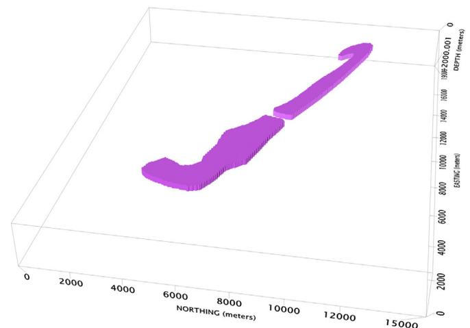
Fig. 1. Simulated iron-ore formation (pink prisms) with density contrast of  $0.75 \text{ g/cm}^3$ . This model was inspired by geologic interpretations of the iron-ore deposit over the Gandarela syncline in Quadrilátero Ferrífero (Brazil).
