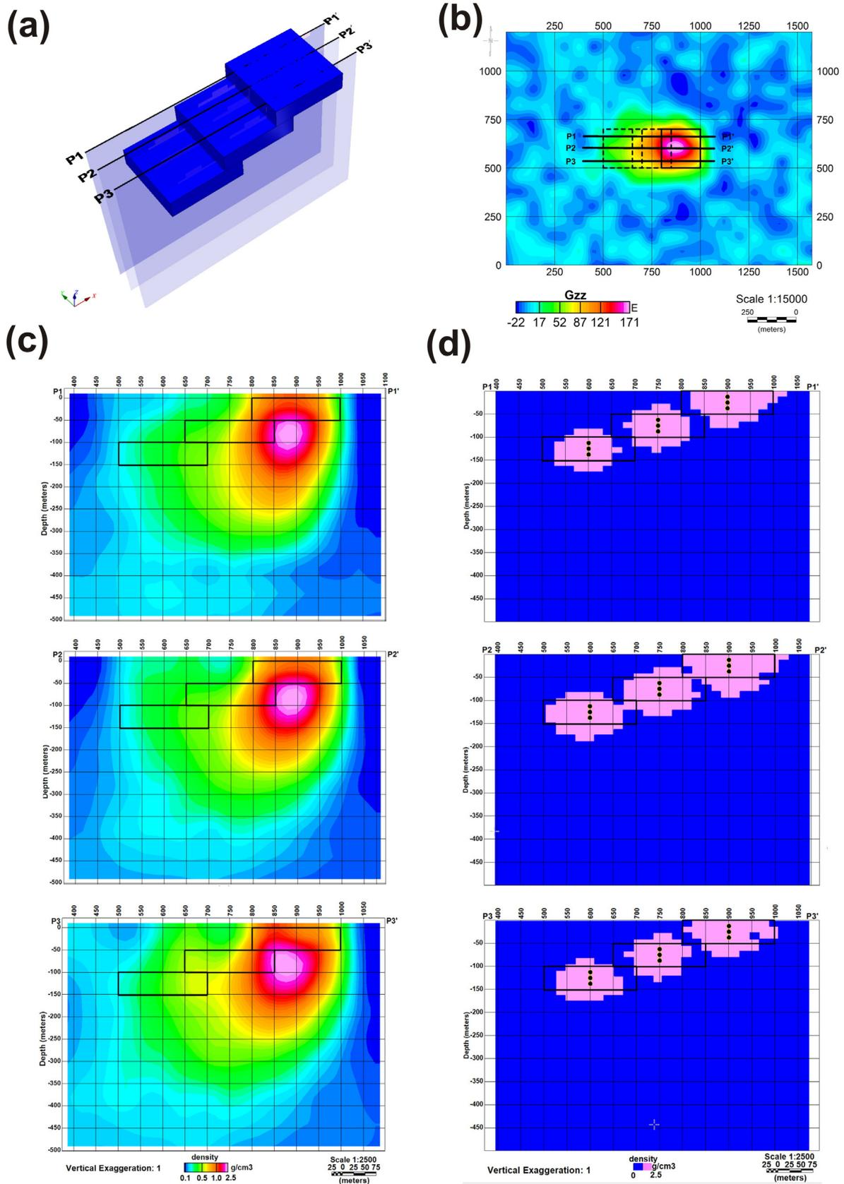
Fig. 7. (a) Simulated dipping body with density contrast of  $2.5 \text{ g/cm}^3$ . (b) Noise-corrupted  $g_{zz}$  — component produced by dipping body shown in (a). Vertical cross sections of the estimated density-contrast distribution produced by (c) the depth-weighting smoothing inversion and (d) the planting anomalous density inversion using a set of seeds (black dots).
